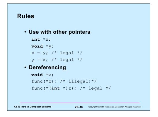
Dereferencing a pointer must result in a value with a useful type. "void" is not a useful type.
