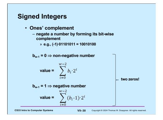
In ones' complement, a number is positive if its leftmost bit is zero negative otherwise. We negate a number by complementing **all** its bits. Thus, if the leftmost bit is zero, a one in position **i** of the remaining bits contributes a value of  $2^{i}$  and a zero contributes nothing. But if the leftmost bit is one, a zero in position **i** contributes a value of  $-2^{i}$  and a one contributes nothing.
