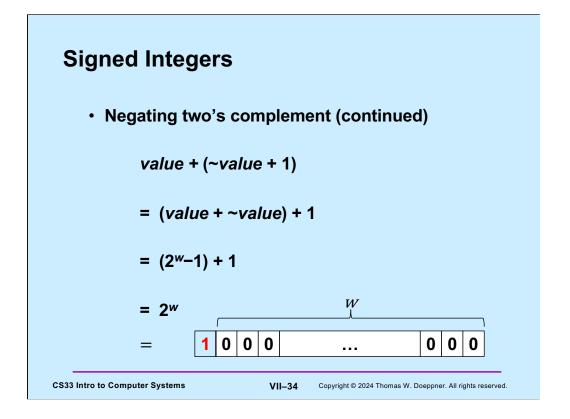
If we add to the two's complement representation of a w-bit number the result of adding one to its bitwise complement, we get a w+1-bit number whose low-order w bits are zeroes and whose high-order bit is one. However, since we're constrained to only w bits, the result is a w-bit value of all zeroes, plus an overflow. If we ignore the overflow, the result is zero.
