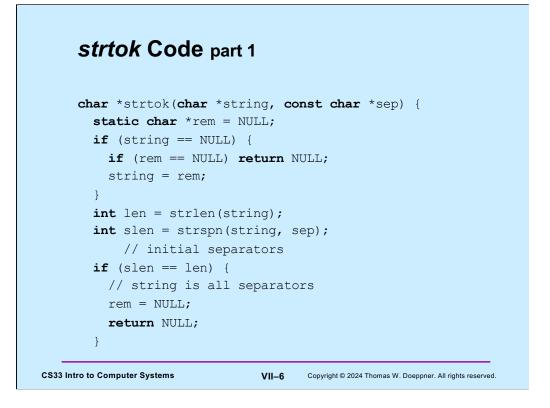
Note the static declaration of **rem** – this allows **strtok** to keep track of the remaining portion of the string.
