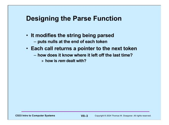
The parse function must keep track of where it left off after each call to it. One way of doing this is via the use of a static local variable.
