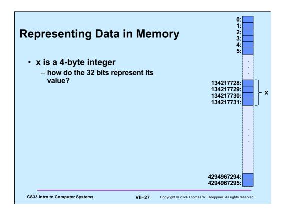
In the diagram, x is an int occupying bytes 134217728, 134217729, 134217730, and 134217731. Its address is 134217728; its size is 4 (bytes).
