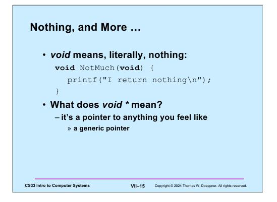
The **void** \* type is an exception to the rule that the type of the target of a pointer must be known.
