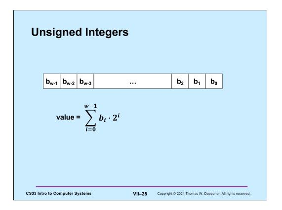
If a computer word is to be interpreted as an unsigned integer, we can do so as shown in the slide, where w is the number of bits in the word.
