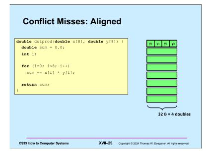
If arrays x and y have the same alignment, i.e., both start in the same cache set, then each access to an element of y replaces the cache line containing the corresponding element of x, and vice versa. The result is that the loop is executed very slowly — each access to either array results in a conflict miss.
