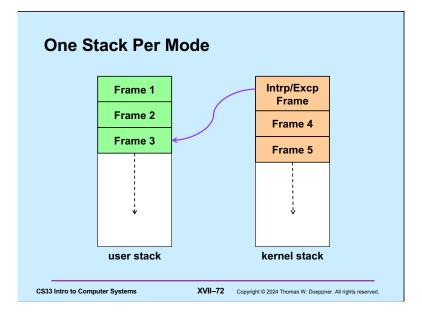
When a trap or interrupt occurs, the current processor state (registers, including RIP, condition codes, etc.) are saved on the kernel stack. When the system returns back to the interrupted program, this state is restored.
