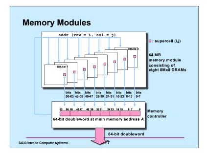
The memory controller pulls in eight supercells from eight DRAM modules and transfers them to the processor over the memory bus.
