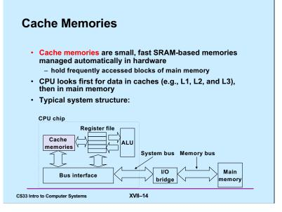
"ALU" (arithmetic and logic unit) is a traditional term for the instruction and execution units of a processor.
