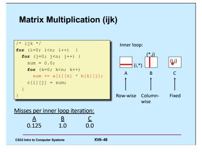
Assume we are multiplying arrays of doubles, thus each element is eight bytes long, and thus a cache line holds eight matrix elements. The slide shows a straightforward implementation of multiplying A and B to produce C.
