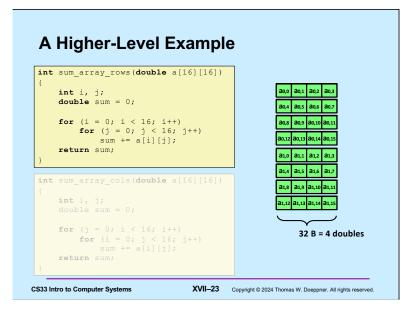
Note that the cache holds two rows of the matrix; each cache block holds four doubles. When a[0][0] is read, so are a[0][1] through a[0][3]. Thus, after one cache miss, we get three hits.
