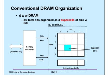
Note that the chip in the slide contains 16 supercells of 8 bits each. The supercells are organized as a 4x4 array.
