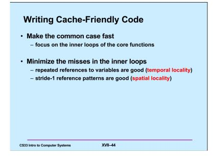
"Stride n" reference patterns are sequences of memory accesses in which every nth element is accessed in memory order. Thus stride 1 means that every element is accessed, starting at the beginning of a memory area, continuing to its end.
