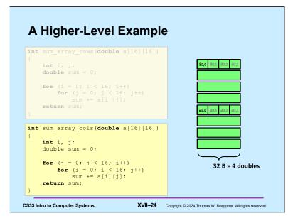
For each reference to an element of the matrix, its entire row is brought into the cache, even though the rest of the row is not immediately used.
