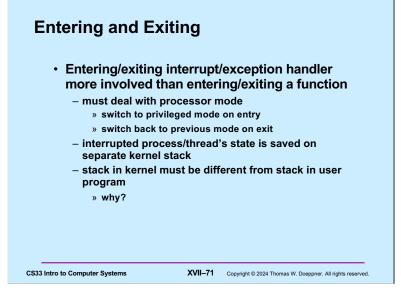
The reason why there must be a separate stack in privileged mode is that the OS must be guaranteed that when it is executing, it has a valid stack, and that the stack pointer must be pointing to a region of memory that can be used as a stack by the OS. Since while the program was running in user mode any value could have been put into the stack-pointer register, when the OS is invoked, it switches to a pre-allocated stack set up just for it.
