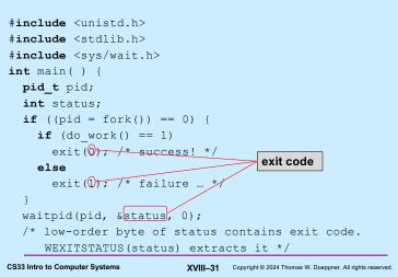
The exit code is used to indicate problems that might have occurred while running a program. The convention is that an exit code of 0 means success; other values indicate some sort of error. Note that if the main function returns, it returns to code that calls exit; thus, returning from main is equivalent to calling **exit**. The argument passed to **exit** in this case is the value returned by main.
