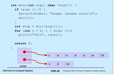
Note that argv[0] is the name by which the program is invoked. argv[1] is the first "real" argument. In this program, argv[2] will contain the NULL pointer (0). argc is two, indicating two arguments (argv[0] and argv[1]).
