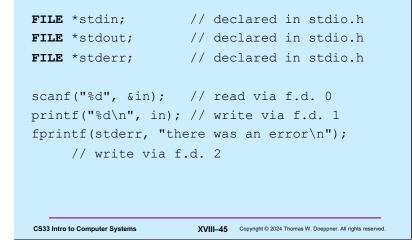
The **streams** stdin, stdout, and stderr are automatically set up to refer to data from/to file descriptors 0, 1, and 2, respectively.
