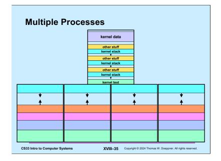
Each process has its own user address space, but there's a single kernel address space. It contains context information for each user process, including the stacks used by each process when executing system calls.
