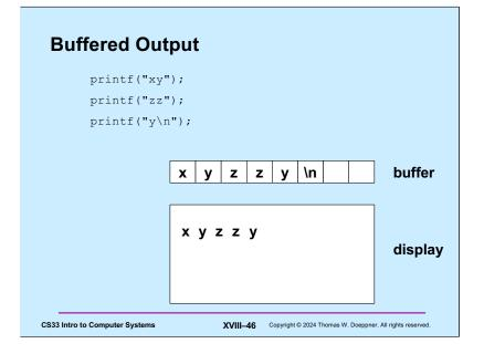
The **stdout** stream is buffered. This means that characters written to **stdout** are copied into a buffer. Only when either a newline is output or the capacity of the buffer is reached are the characters actually written to the display (via a call to **write**). The reason for doing things this way is to reduce the number of (relatively expensive) calls to **write**.
