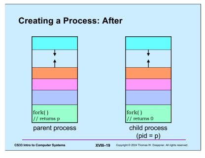
By executing **fork** the parent process creates an almost exact clone of itself that we call the child process. This new process executes the same text as its parent, but contains a copy of the data and a copy of the stack. This copying of the parent to create the child can be very time-consuming if done naively. Some tricks are employed to make it much less so.
