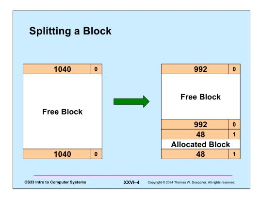
Splitting a block is straightforward. We take a block that was previously free and divide it into two blocks – an allocated block that's big enough to hold the storage request, and the remainder represented as a free block.
