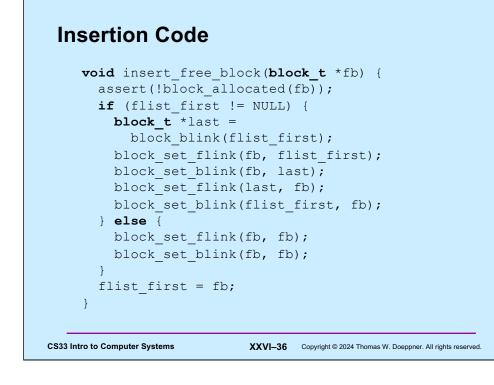
Using our functions, here's the code to insert a block at the beginning of the free list.
