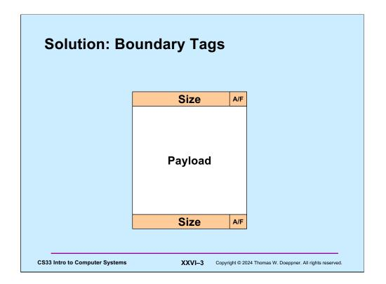
One solution (which we use in the malloc assignment) is the boundary tags approach. Here we have a fixed overhead for each block of memory (whether free or allocated) that indicates its size and whether it's free. So that we can determine if adjacent blocks are free (and what their sizes are), we put this information at each end of the block. The non-overhead portion of the block (which is available to hold data) is called the **payload**.
