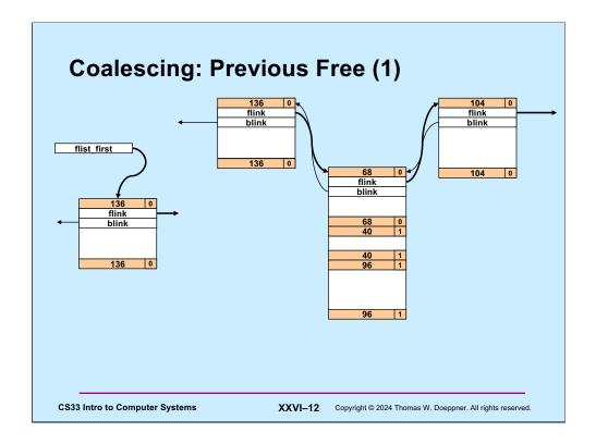
Suppose the previous block is free, but the next block is allocated. Thus, the previous block is in the free list. We'll assume it's not the first element of the free list, which is pointed to by **flist\_first**.
