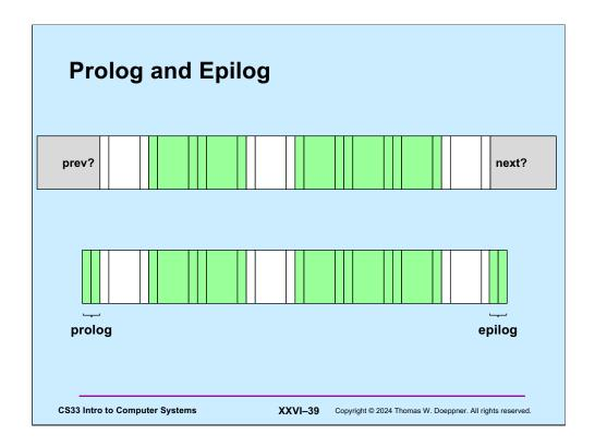
The slide shows our heap, with allocated blocks shown in green and free blocks in white. At either end of each block are its tags.
