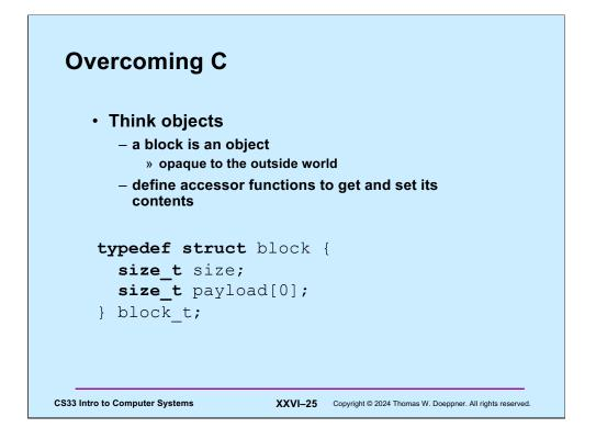
Putting a zero for the dimension of payload is a way of saying that we do not know a priori how big payload will be, so we give it an (arbitrary) size of 0. Note that sizeof(size\_t) is 8 (i.e., **size\_t** is a typedef for a **long**).
