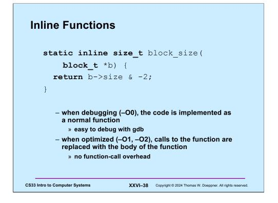
If we declare a function to be **inline**, the C compiler is instructed to replace calls to the function with its actual code (unless -O0 is specified). Thus, inlined functions have no function-call overhead (though they do increase the total size of our code, which does come at some cost).
