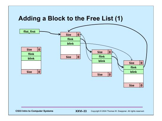
An important operation is to add a block to the beginning of the free list. We start with a picture of the free list.
