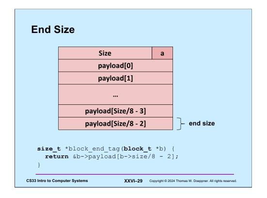
The block\_end\_tag function returns the address of a block's end tag, given the address of the beginning of the block (where its front tag is).
