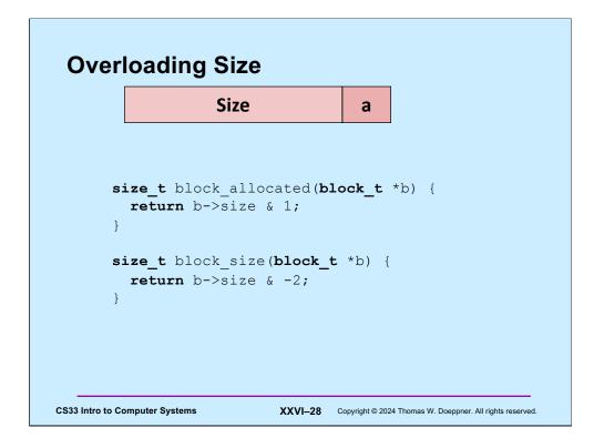
If we assume that the size of a block is always even (in practice it's probably a multiple of 4 or 8), then we can assume the least significant bit is zero and use that bit position to represent the allocated flag.
