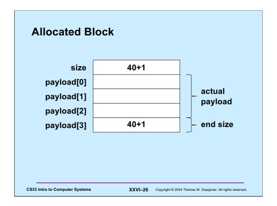
In this example we have an allocated block of 40 bytes. Its size and end size fields have their low-order bits set to one to indicate that the block is allocated. (Since each element of payload is 8 bytes long, the entire allocated block, including tags, is 40 bytes long.)
