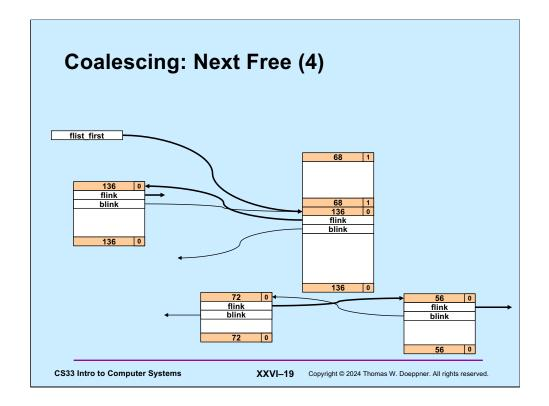
Finally, we insert the combined block into the beginning of the free list.
