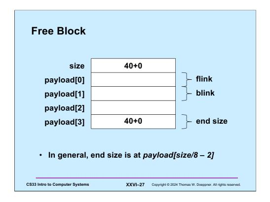
For a free block, the size fields contain the exact size of the block: the allocated bits are zeroes. The first two elements of payload are the flink and blink pointers, respectively.
