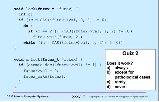
In this version, if the futex's value is 0, it's unlocked, if it's one it's locked and no threads are waiting for it; if it's greater than one it's locked and there might be threads waiting for it.
